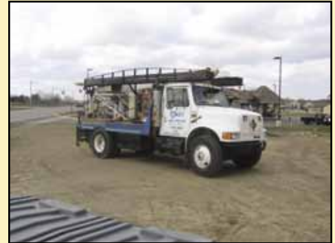
IHC 4900 Pump Hoist
